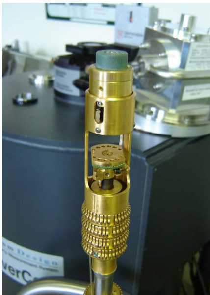
Figure 2.6 One of the sample platforms available to hold the sample puck. | Source: Properties of Materials: Physical Property Measurement System (PPMS) Institute for Research in Materials (IRM) Dalhousie University |
