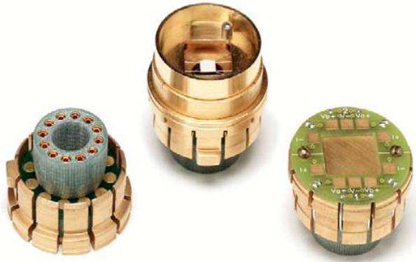
Figure 2.5 (left) 12 pin connection; (middle) heat capacity microcalorimeter puck; (right) AC transport puck | Source: Properties of Materials: Physical Property Measurement System (PPMS) Institute for Research in Materials (IRM) Dalhousie University |
