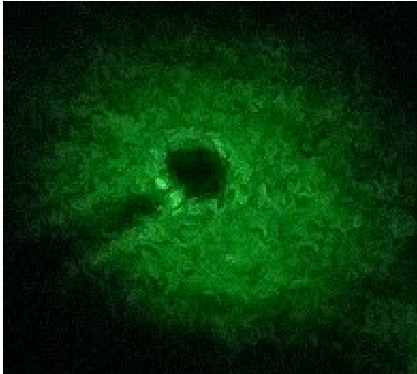
Fig. 2.10.: Generated LG beam from microscope cover slip
