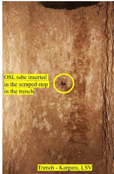
Figure 31. OSL sample collection from step-trench at Kargara.
