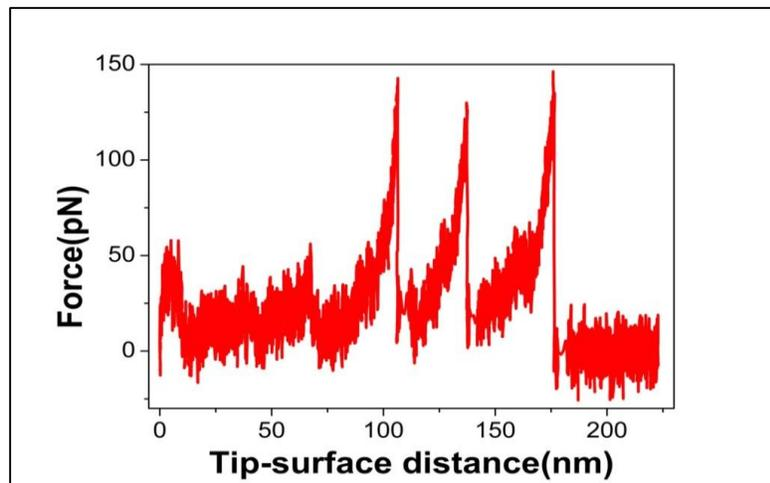
**Fig. 3K: Force curve: saw tooth pattern of force curves indicating force vs extension profile showing unfolding of three domains.**
