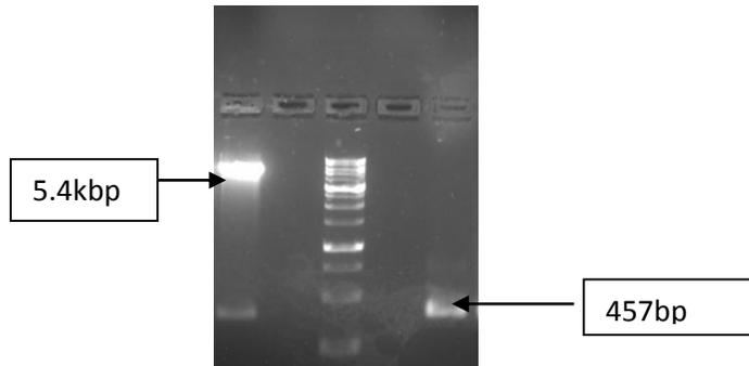
**Fig.3F: Digestion of the vector and insert for the EC1 monomer with GGG**
