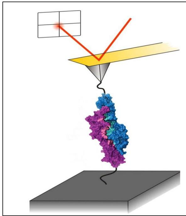
**Fig.1C: Picture demonstrating Force Spectroscopy study using AFM**
