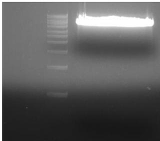
The cut vector is shown on the left. The digestion of the insert is not run in gel and instead purified directly using Invitrogen's DNA Purification Kit. The pre-ligation check is shown below.
