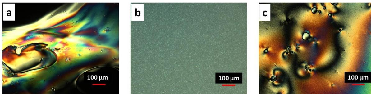
**Figure 4.1** POM microphotographs of the optical texture of lamellar phases formed by (a) **F-5** at 66 °C, (b) **F-7** at 53 °C, (c) **F-9** at 60 °C, observed on cooling with a rate of 5 °C min<sup>-1</sup>.
