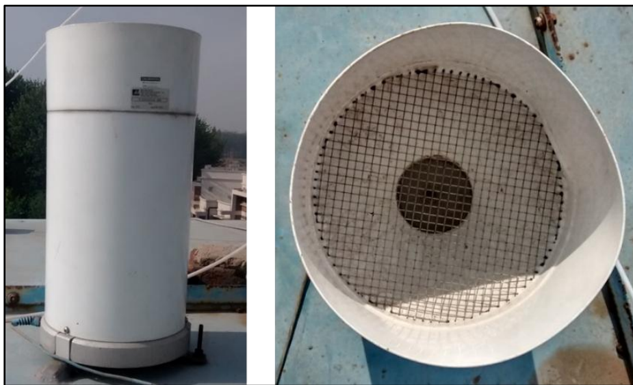
Picture 2.2: Picture of the tipping bucket rain gauge installed at the top of the atmospheric research facility at IISER Mohali.
