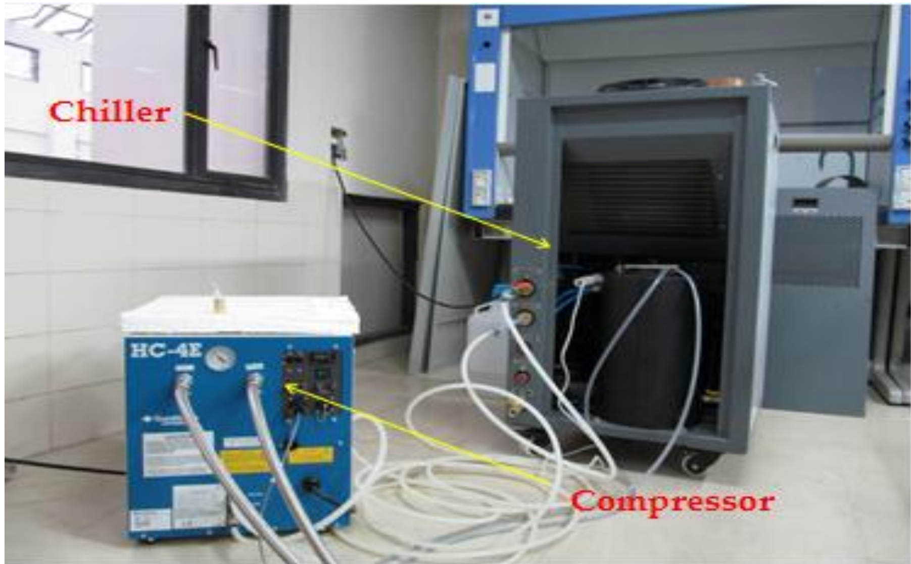
Figure 6. Photograph of Compressor and Chiller
