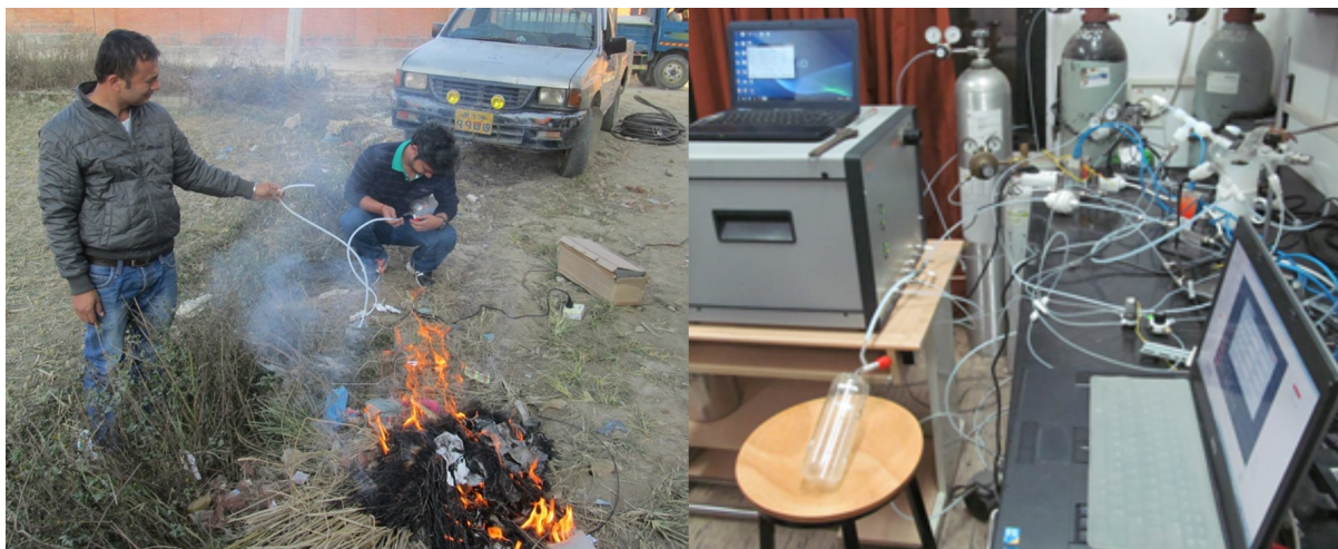
Figure 5.7: Collection of garbage burning grab samples in the Kathmandu Valley (on left) and the instrumental setup for the analysis (on right)
