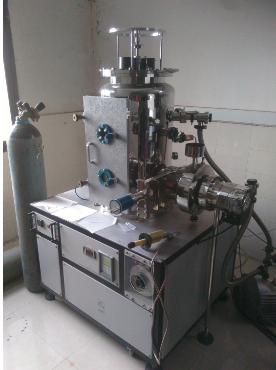
Figure 3.8: E-Gum Evaporator (this instrument is used for depositing thin film, mostly high melting point materials are used)
