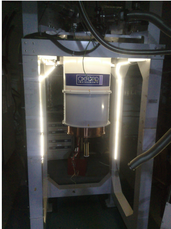
Figure 3.14: Dilution Refrigerator (this instrument is used to cooling the sample)
