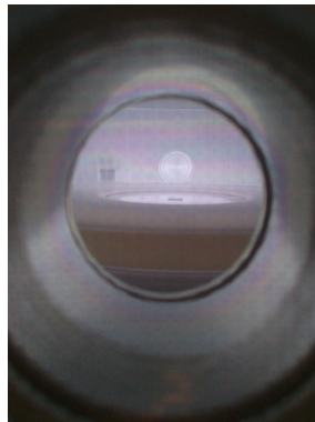
Figure 2.14: SF6 plasma inside plasma etching machine.
