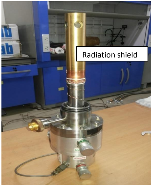
Fig 2.2: Cold head with sample holder, radiation shield
