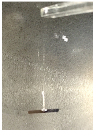
Figure 3.1: Torsion Pendulum made using a silk thread as the suspending thread.
