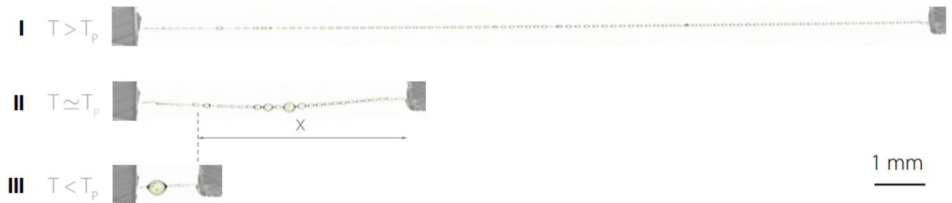
Figure 3.10: Spooling action in Araneus Neoscona capture silk[ref]. At (I), the spring in this state behaves like a spring. At (II), the tension is decreased, the spooling action begins. At (III), almost whole length of capture is spooled inside a single motifs of capture silk [4].
