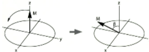
Figure 1.6: magnetisation flip due to application of RF pulse[32].
