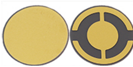
FIGURE 2.3: 6MHz AT-cut quartz.
