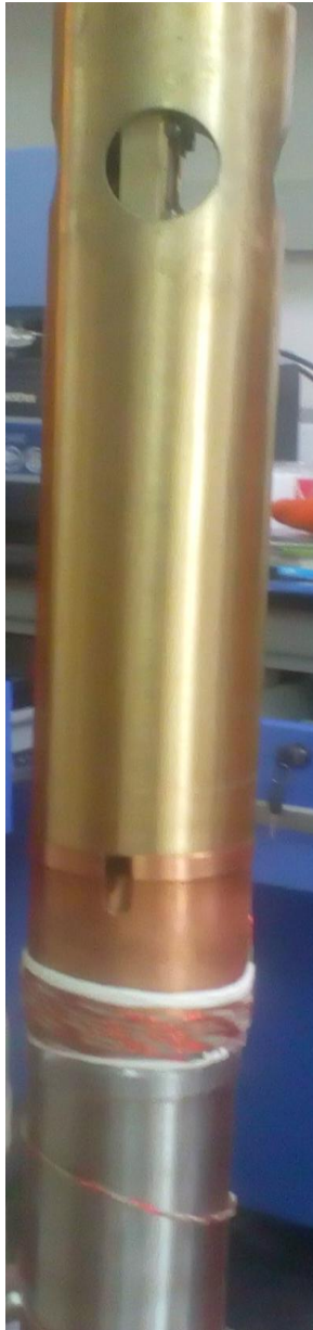
Fig. 2.2: Radiation shield of the cryostat
