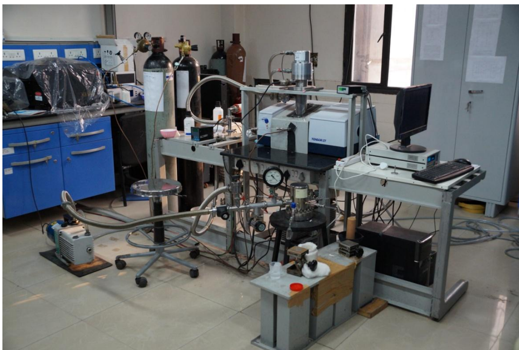
Fig. 2.6: The MI-FTIR setup at IISER Mohali
