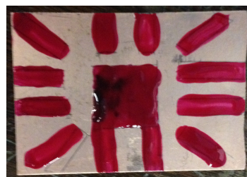
Figure 5.11: Nail-polish set into PCB in desired shapes for making contact pads
