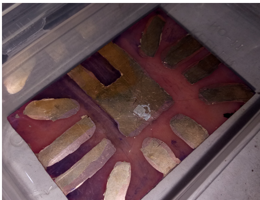
(a) LAO-STO sample wirebonded in a PCB
