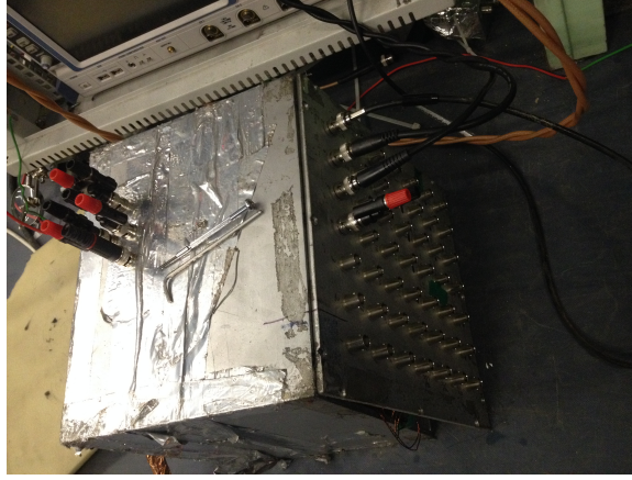
Figure 4.5: A break-out box with some grounding caps connected to it
